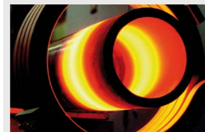
Inductively heated pipe
